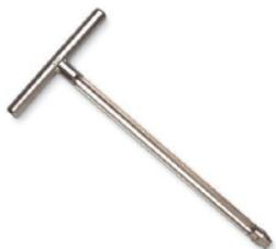
**LEFT:** A soil probe makes pulling samples easy. Stop by the office to borrow one of ours "free of charge".
