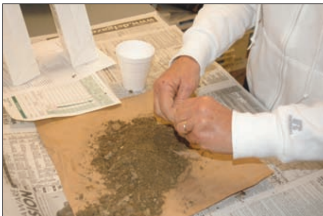
Figure 8. Air dry the sample overnight, break up the clumps, and make a composite sample. Photo credit: Gary Gao.
