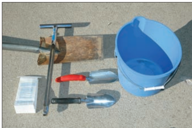
Figure 5. In addition to a soil probe, a spade, knife, or trowel can also be used to take thin slices or sections of soil. Photo credit: Gary Gao.
